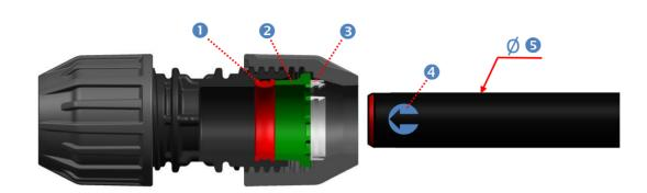
High Tolerance type is available for sizes ½", ¾" & 1". The breakthrough designed fitting seals pipes with in-range external diameter. Furthermore the same fitting can be installed on pipes as defined by several standards (IS134, BS1972, etc.).
