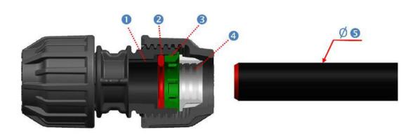
Kit type is available for Normal Gauge pipes of IS134 with nominal size ½", 1 ¼", 1 ½" & 2". The existing metric compression fittings can be converted to imperial fittings by substituting the metric O-ring, insert and split ring with the relevant Agriflow KIT (sleeve insert, rubber seal, insert and split ring).
