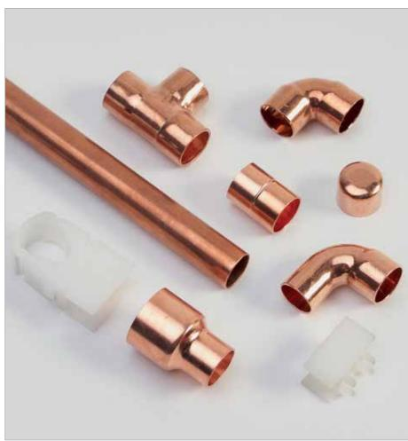
End Feed fittings are used for connecting copper piping and provide a robust yet, economical option. Copper piping and joins are suitable in plumbing applications for both hot and cold water supplies. Connections are made by applying flux and a heat source to reach a suitable temperature, then adding solder around the joint to seal
