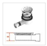
GW90 Metal Topped 90mm diameter waste provides a high rate 27 l/min when installed with a 15mm head and 1m pipe installation
