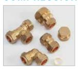
Compression Fittings are used to couple together pipes or to connect a pipe to a fixture or valve. There are three elements to a compression fitting: a nut, ring and seat. These work together to give a watertight connection. This simple mechanism makes it quick and easy for installers to connect or disconnect fittings.
