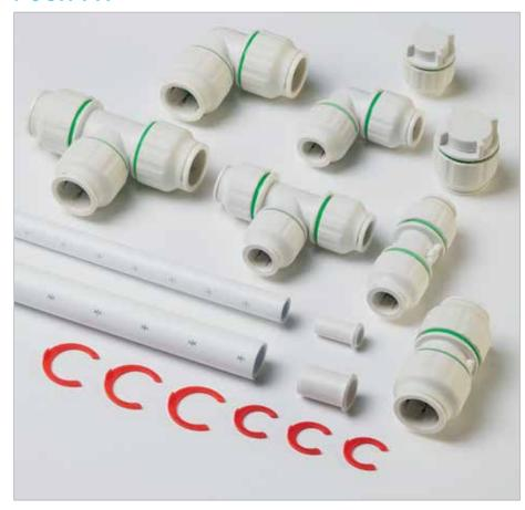
Push Fit plumbing fittings are quick and easy for installers to connect without the need for any specialist tools or sealant. Push Fit works by inserting the pipe into the fitting and then sealing a watertight connection by twisting the rotating sealing cap. Unlike with some other fittings, Push Fit connections can be disassembled and reused by twisting the sealing cap on the fitting. Our Push Fit range comes from industry leading brands to ensure quality and reliability.
