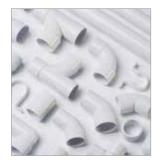
Solvent Weld pipes and fittings use solvent cement to create a permanent joint. Solvent cement is brushed to the inside of the fittings and the outside of the pipe, then the pipe is inserted into the fitting and twisted to ensure full coverage. Solvent Weld waste pipe and fittings are used to connect appliances to the waste network in the building that carry it away. Our Solvent Weld range comes from Floplast, a brand with a strong reputation for quality and reliability.
