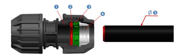
Kit type is available for Normal Gauge pipes of IS134 with nominal size ½", 1 ¼", 1 ½" & 2". The existing metric compression fittings can be converted to imperial fittings by substituting the metric O-ring, insert and split ring with the relevant Agriflow KIT (sleeve insert, rubber seal, insert and split ring).
